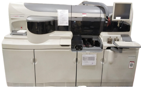
Vistro 5600 Chemical Analyzer is indeed used for a comprehensive range of biochemistry and hormonal tests, including Blood Sugar, Liver Function Tests (LFT), Renal Function Tests (RFT), Lipid Profile, and Thyroid Function Tests.
