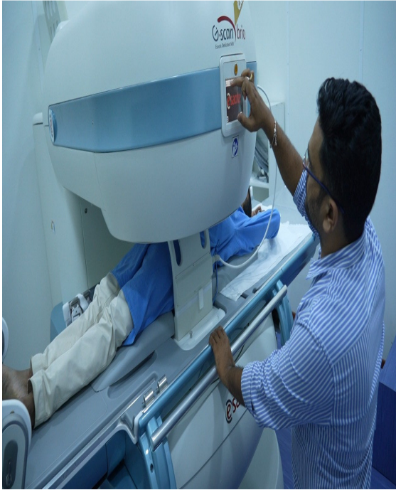
Open MRI to scan Clustrophobic Patients.
