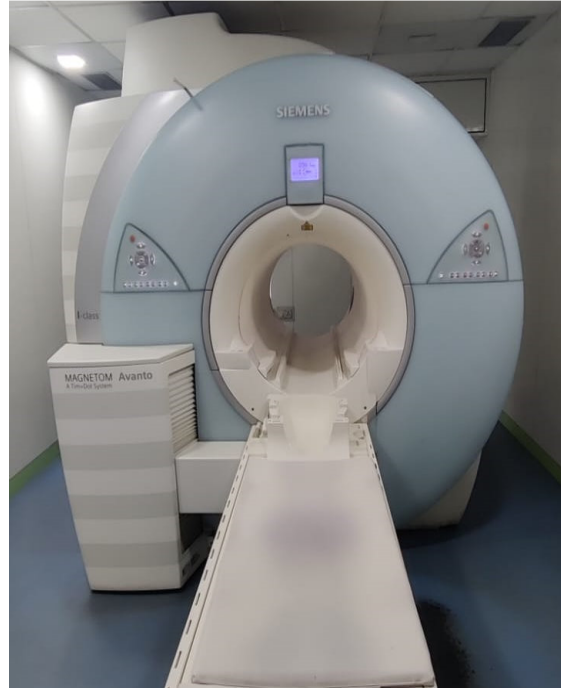
High Field MRI to get High Resolution Image
